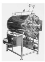
controller, which controls pressure and temperature with temperature indication, factory set at 121° C (15 PSI), along with built in digital timer adjustable for maintaining Sterilization cycle time with auto cut off. # Fully Automatic Model: Temperature automatically maintained by digital controller, which controls / pressure and Temperature with auto air purge, digital timer, auto steam exhaust, low water level cutoff.
